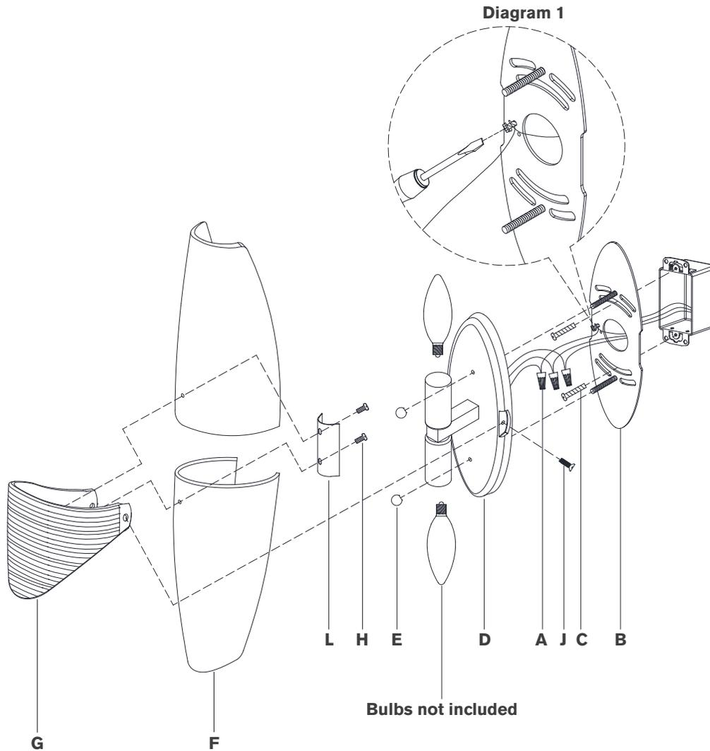
10. Install glass (F) to cap (G), securing with metal plate (L) and screws (H).
