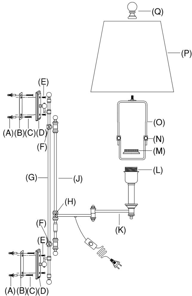
1. Position fixture bases (D) to the wall in desired orientation and use it as a template, mark outlet line for both fixture bases (D) on the wall. Remove the fixture base.
