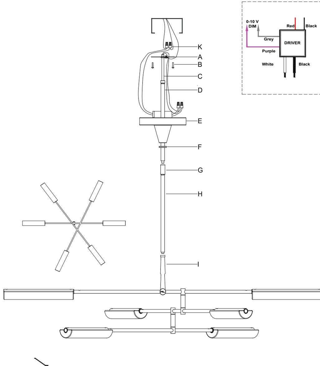
12. Connect the driver input black wire to the hot wire in the junction box using the wire nut (K).
